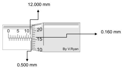
sleeve reads full mm = 12.000sleeve reads half mm = 0.500thimble reads mm = 0.160
